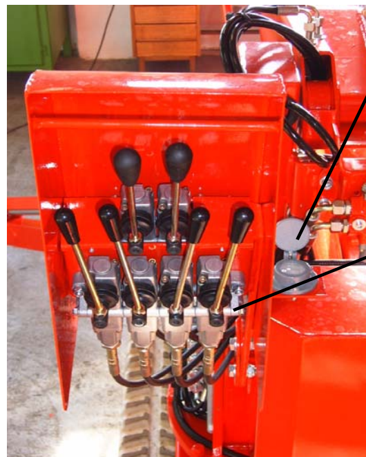
11. Selection switch: Position of stabilizing (quick moving)
