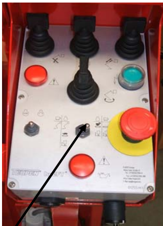
11. Selection switch: Position of stabilizing (quick moving)
